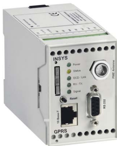
Figures 1,2: GPRS data communication devices: INSYS GPRS 5.0 and i-module GPRS 3.0 (right)
