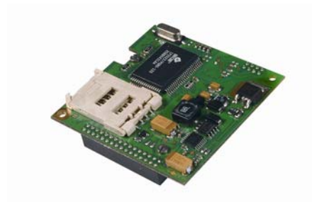
Figures 1,2: GPRS data communication devices: INSYS GPRS 5.0 and i-module GPRS 3.0 (right)
